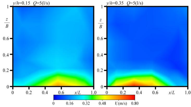
Fig. 4 Contour of flow velocity in vertical section
