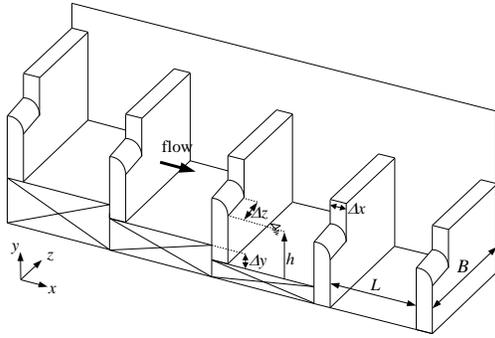
Fig. 1 Pool-and-weir fishway
